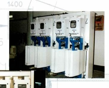
In-line filling machines with one or up to four modules, alternatively with vertical or overhead bag drop.
